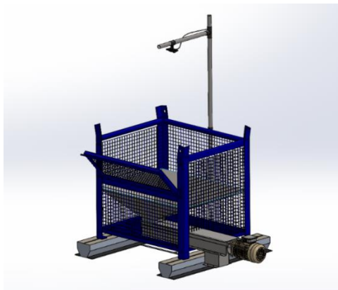
Figure 2.8. Integrated system for input control. Smart chest (D)
