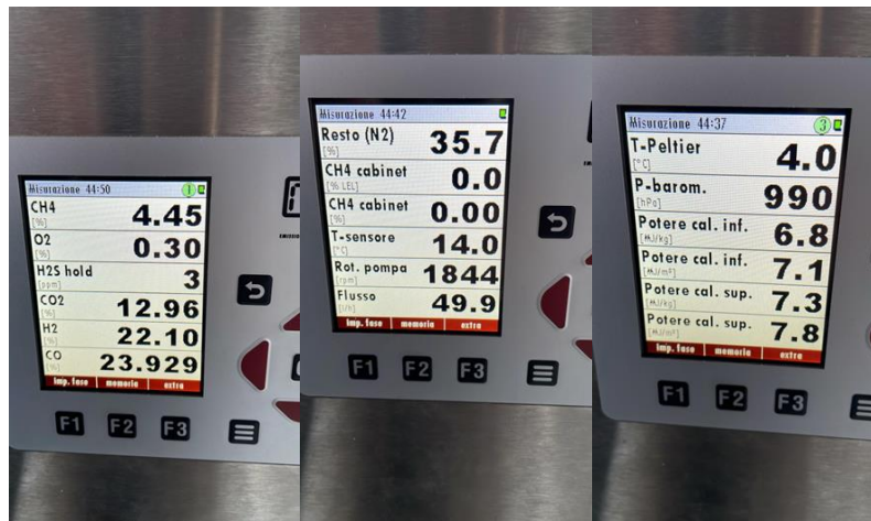
Figure 1.2. data taken with Green plasma system SWG100 MRU test.
