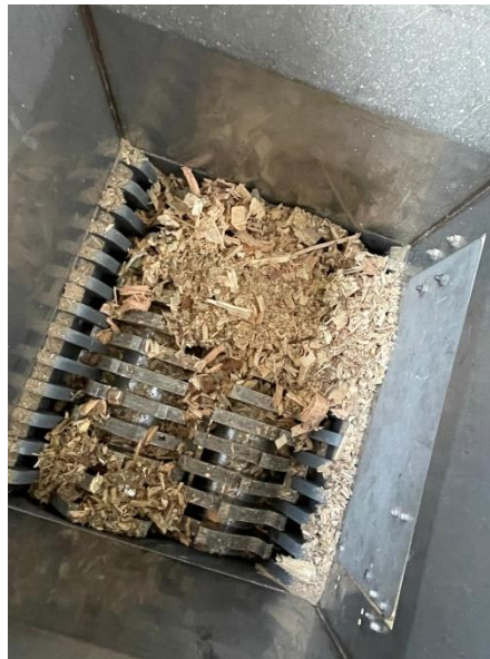
Figure 2.2. Woodchip being shredded.
